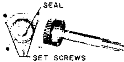
Fig. FO38—Clutch shaft and bearing assembly can be removed from front support after loosening Allen screws in support.
